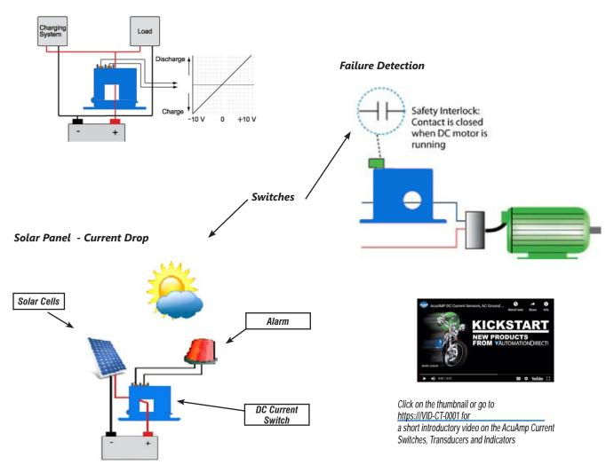
When the sun is blocked, the current drops. The Current Operated Switch detects the drop in current and activates the relay which turns on the alarm light.
