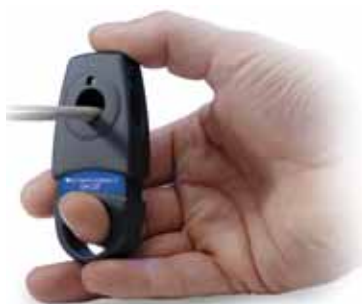
DN-CST Precision Stripping Tool [squeeze, insert cable, rotate, & remove]
