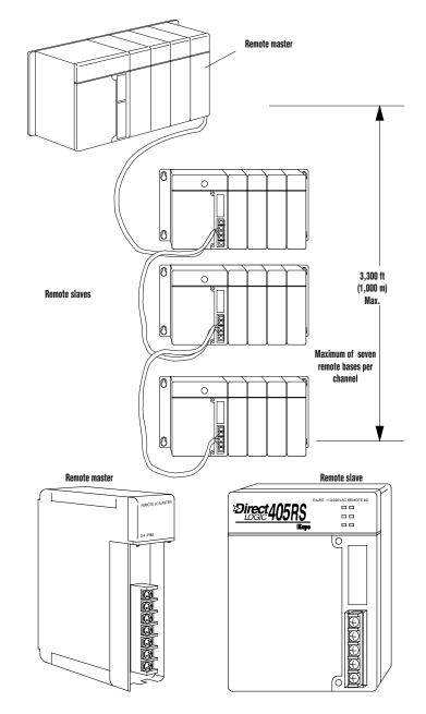
You can assign normal input and output addresses to the remote points, or you can assign special remote I/O addresses. The Remote Master sends the remote I/O information to the CPU. The communication between the Remote Master and the CPU is asynchronous to the CPU scan. For this reason, remote I/O applications should be limited to those that do not require the remote I/O points to be updated with every CPU scan.
