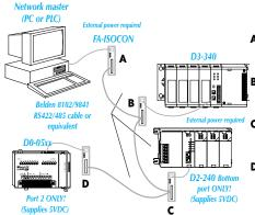
A) FA-ISOCON converts the network master's (computer or PLC, etc.) RS-232 communication signal levels to RS-422/485.
