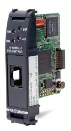
The HO-ECOM100 supports the Industry Standard Modbus TCP **Client/Server Protocol**
