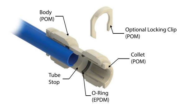
Push-to-Connect Fitting Cut-away Diagram
