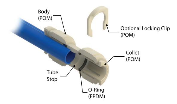
Push-to-Connect Fitting Cut-away Diagram
