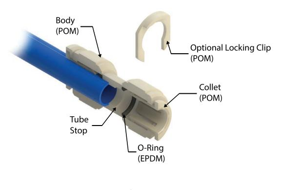
Push-to-Connect Fitting Cut-away Diagram
