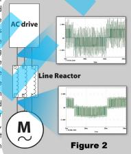
spikes going from the drive to the motor. Line reactors are used in many instances when the motor is located far from the drive [see Figure 2].
