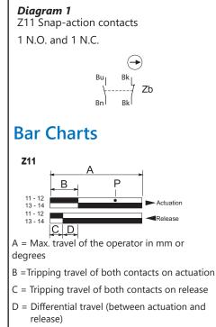
P = Point from which positive opening is assured during actuation
