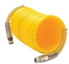
NITRA™ nylon coiled hose is an excellent choice for industrial environments requiring higher working pressure and higher temperature/ chemical resistance. Manufactured from Nylon 12, these hoses include spring guards to resist kinking and have male nickle-plated brass NPT swivel fittings on each end.
