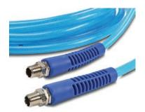
NITRA<sup>™</sup> reinforced polyurethane (PUR) hose features a sturdy polyester braid between the polyurethane inner and outer layers. Contamination of air systems caused by rubber hose breakdown is significantly reduced by using NITRA PUR hose. CBL2 and CBL3 hoses have one rigid and one swivel fitting and are specified by inside diameter. CBL5 and CBL6 hoses have one Male and one Female industrial interchange quick disconnect fitting.
