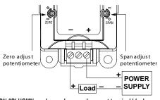
DN-3PLUGMN can be used as a replacement terminal block.
