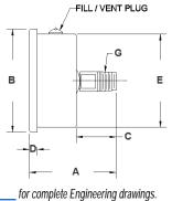
**Dimensions - Lower Mount Gauge** A 2.190" [55.6 mm] В 2.700" [68.5 mm] С 0.433" [11.0 mm] D 0.250" [6.3 mm] Ε 2.440" [61.9 mm] F 1.035" [26.3 mm] G 1/4" NPT 0.551" [14.0 mm] Η
