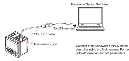
When using the maintenance port, power is provided from the USB port. Do not supply power to the controller through the terminals until disconnected from the maintenance port.
