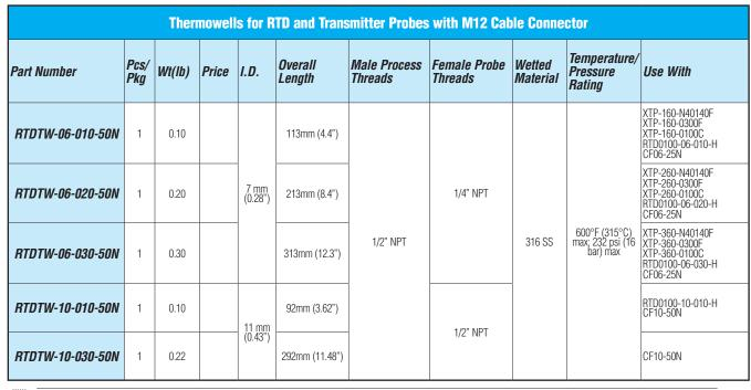
Note: Check the chemical compatibility of the thermowell's wetted parts with the medium to be measured.
