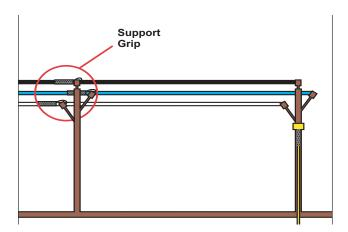
CAUTION: Never use grip to approximate breaking strength. Refer to technical data page for safety and working load factors. Banding is necessary to guard against accidental release of grip and provide maximum reliability.
