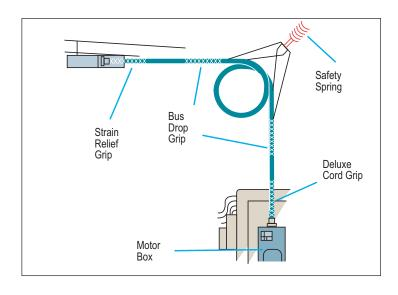
CAUTION: Never use grip to approximate breaking strength. Refer to technical data page for safety and working load factors. Banding is necessary to guard against accidental release of grip and provide maximum reliability.
