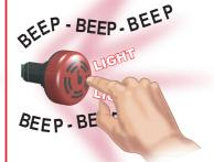
The audible signal can be silenced quickly by lightly pressing on the front of the indicator.
