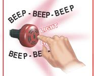
The audible signal can be silenced quickly by lightly pressing on the front of the indicator.
